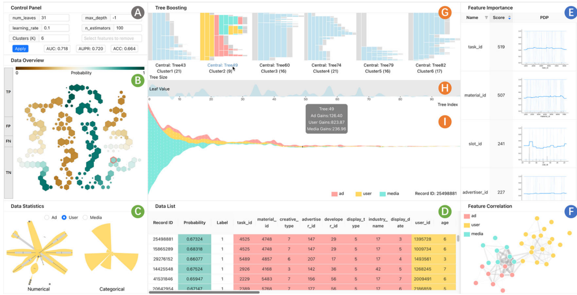
Fig. 1 The user interface of GBDT4CTRVis. GBDT4CTRVis assists advertising analysts in understanding the working mechanism of the GBDT-based CTR prediction model on multiple levels and facilitating the model tuning process. (1) Instance level: explore the prediction results of advertising data instances hierarchically through data overview (B), data statistics (C), and data details (D). (2) Feature level: analyze the importance of features (E) and the correlations (F). (3) Model level: display the most representative K decision trees (G), observe the evolution of the tree size (H), and present the evolution of the information gain during the model prediction (I). Analysts can also adjust hyperparameters and evaluate prediction performance through the control panel (A)
